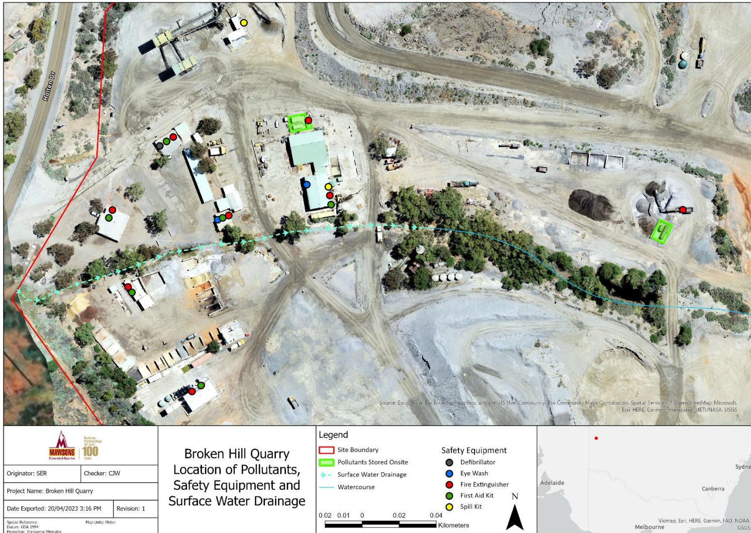
Figure 3: Location of pollutants, safety equipment and surface water drainage onsite
